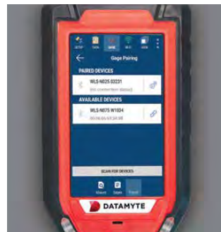
Automatically detect, display serial number, and use correct gauge as characteristic's data source
